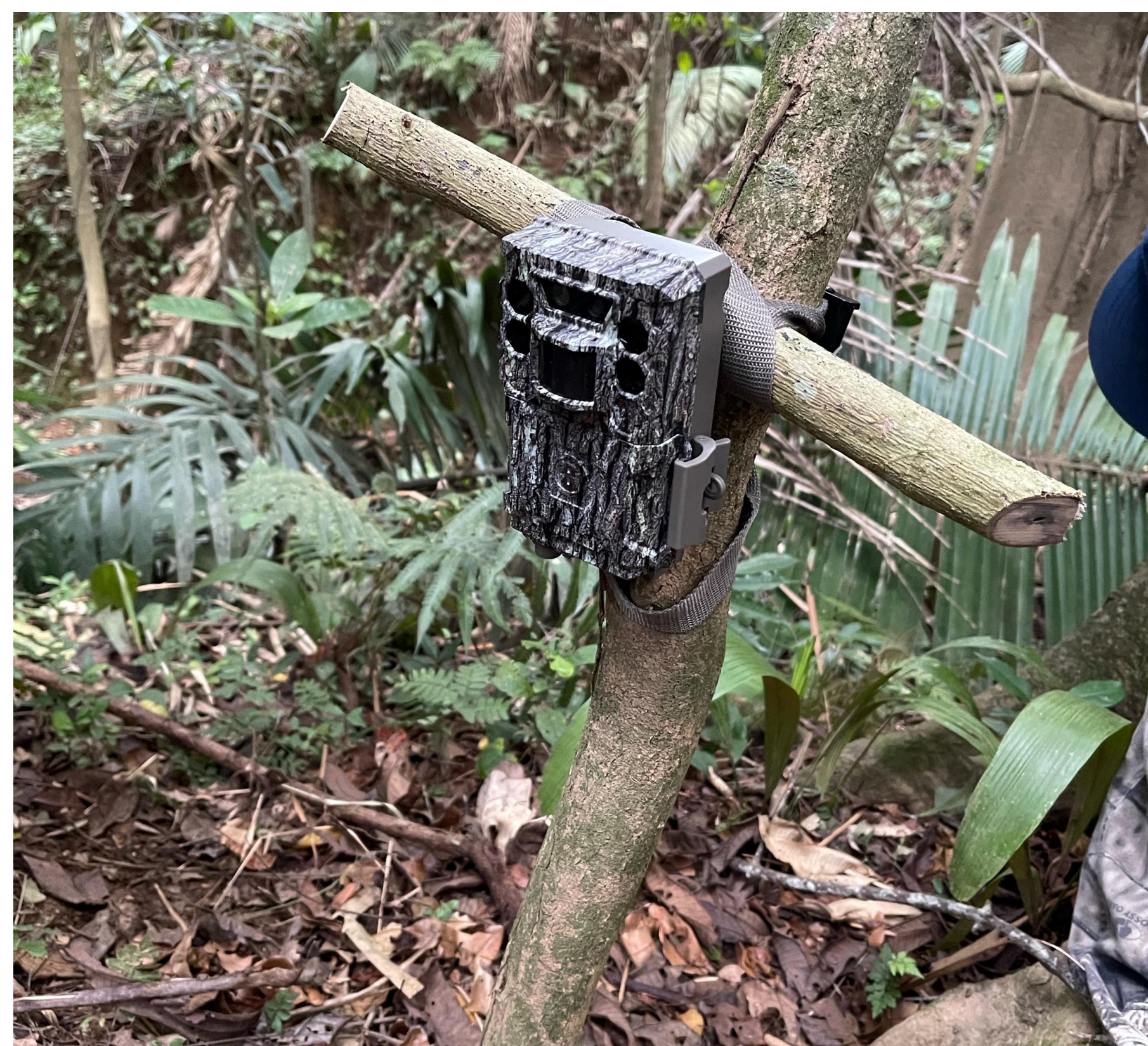
Figure 2. One of the camera traps used in the study immediately after installation. Picture credit Flor Mucino.
